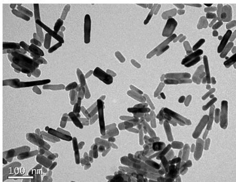
Fig. 1. TEM images of ZnO NR, showing the morphology compatible with NRs on nanoscale.
